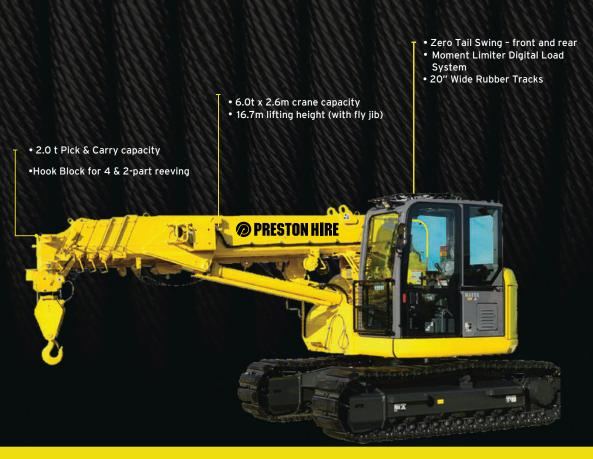
Preston Hire SuperCrane 1485 has a maximum lifting height of 16.7m. This compact crane has a small footprint and because it does not have outriggers, it is ideal for use in tight areas. It boasts a 2.0t pick & carry capability. Other features include an air-conditioned enclosed cab and a machine weight of 14,560kg. Consider the possibilities...
