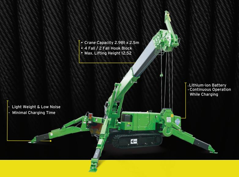
The fully electric-powered Maeda MC305CB mini crane with zero emission, without compromising on performance. Innovative lithium-ion batteries make these models environmentally friendly, economical, efficient, and safe. You can fully operate the crane while charging and short recharge time allows for a more continuous operation. Consider the possibilities...
