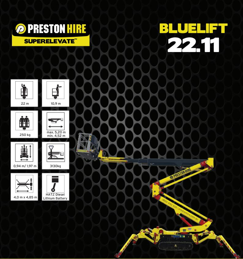
The Bluelift 22.11 is great for larger jobs, offering a maximum vertical reach of 22m, plus an outreach of 11m even with two people in the basket. Variable leg placement comes standard, enabling the unit to be set up in a number of configurations, the narrowest being a leg stance of only 1985mm, which is ideal when units are deployed in driveways, walkways or between buildings.
